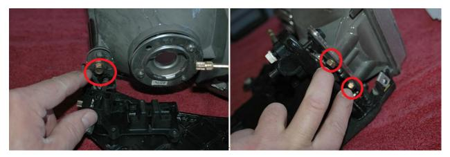
6. For certain year of Corvette, there is bracket rib that will need to grind off to able to clear the projector housing.
