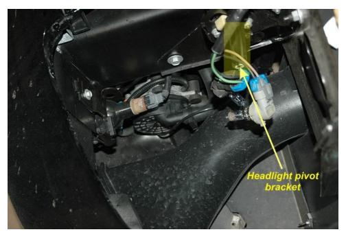
5. Once the headlight removed, losing 3 screws at the headlight bracket to separate the light housing.
