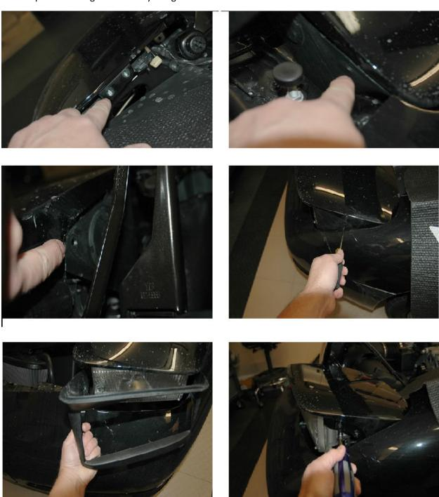
3. Remove the headlight assembly by losing two rear pivot screws
