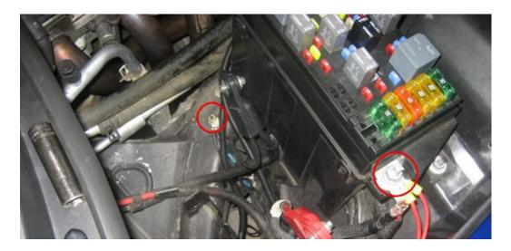
8. Connect the Headlight wiring harness as picture below.
