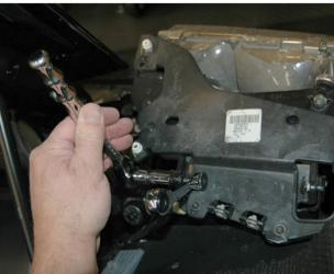
4. Remove the locking pin underneath the headlight housing that attached to the motor.
